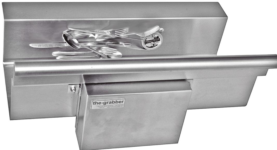
A focused magnetic retrieval system within a 16 gauge 300 series stainless steel water resistant sealed housing and mounting flanges. Each system consists of a pair, one **the-grabber** magnet unit mounted on each side of a trough.
